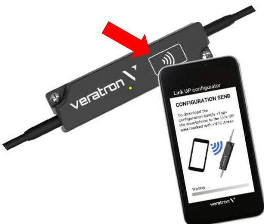
1. Launch the “Link Up Configurator” App and read the actual configuration of the LinkUp device by “tapping” the smartphone onto the devices wireless area (indicated by the red arrow).
