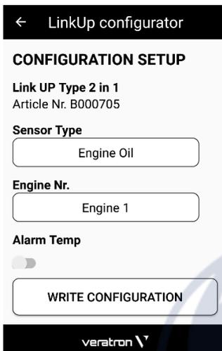
3. As a first step, choose your sensor type out of the options in the first box. (Sensor for engine oil or transmission oil)
